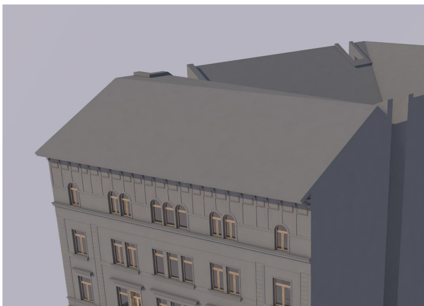
Example of a roof truncated by a near-horizontal plane that does not appear on the façade
